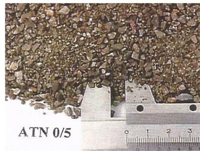
Crushing natural sand 0 mm-5mm
