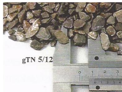
Crushing natural gravel 5mm-12mm
