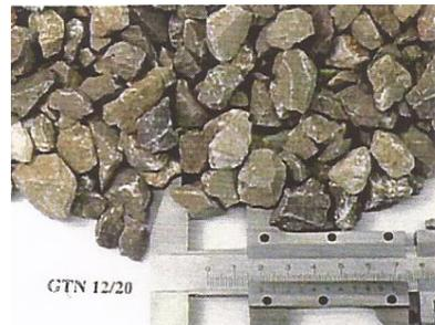
Crushing natural gravel 12mm-20mm
